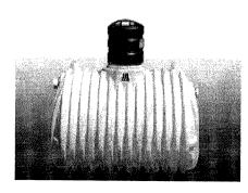
Supply one (1) Mercer International, Inc. *Compliance Master* oil/water separator, Model MI-B25-PE rated at 5-25 gpm. Unit is a cylindrical, gravity-displacement, high-density polyethylene separator tank with nominal oblong dimensions of 51" wide x 102" long. The following standard features shall be included:
